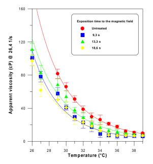
**Fig.4**-Apparent Viscosity of Synthetic Paraffin Solutions versus Temperature for Different Exposition Times (Magnetic Field of  $0.60 \text{ T} @ 40^{\circ}\text{C}$ ).
