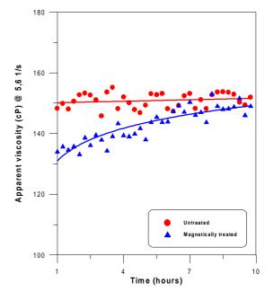
Fig. 3- Apparent Viscosity of Crude Oil Versus Elapsed Time.(Sample: Untreated and Magnetically-Treated at 0.83 T @  $40^{\circ}$ C).
